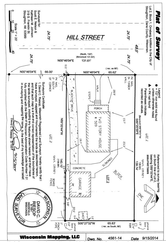
hired after construction, the actual boundary is in fact located 2 feet to the north of this stake, incongruent with existing landmarks. According to this survey, the west end of the garage is 3.7 (a violation of 3.6 in) feet from the property line and the east end is 3.8 feet (a violation of 2.4 in)from the property line.
