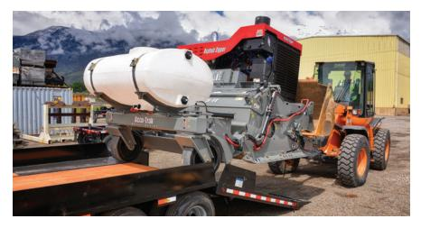
**Custom tandem-axle trailer** (optional) with quick-load guiding system, low center of gravity, convenient working deck and built-in custom toolbox, enables the 720Xi WA to be hauled behind a 2-ton pickup truck.
