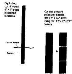
Drill 2 holes in backer boards to accept bolt, washer, nut combo; round all corners and smooth all edges with sandpaper
